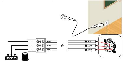
2 Minimize the microphone volume **MIC VOL** before power on. Then adjust to a proper level on demand after power on.
