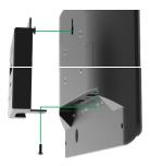
To attach the SYN-TOUCH10, slot the mount key into the keyhole on the back of the tablet and use one of the provided M3L8 screws to secure in place
