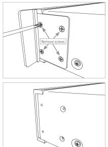
2 Install the rackmount bar ensuring that it aligns with the rackmount holes. The tapered holes of the rackmount bars should be positioned outside and not beneath.
