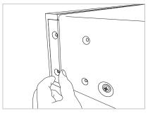
**3** Use the two screws to fix into place the rackmount bar. Use the other two screws to cover up the two vacant screw holes.
