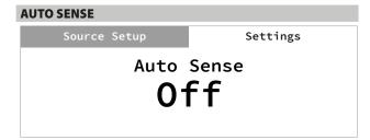
Auto sense feature enables the C 388 to wake up from standby mode when triggered by network connected App or active source input.
