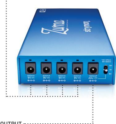
One output provides selectable 9V, 12V, or 18V DC with center negative polarity. It provides 500mA of available current at 9V, 375mA at 12V, and 250mA at 18V. Make sure this output is set to 9V before connecting your Strymon pedals.
