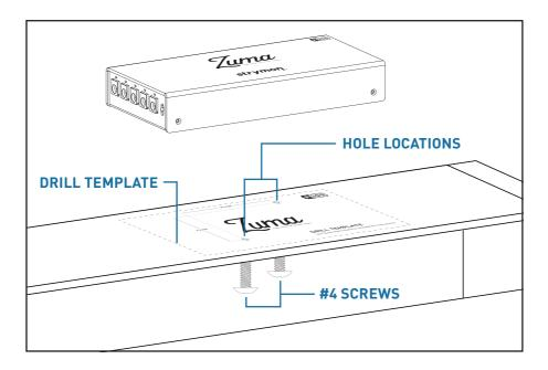
**3** Drill holes. Drill through the two marked hole locations with a 1/8" (3mm) bit. Remove the drilling template.
