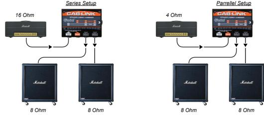
Ensure that both cabinets have the same impedance in Ohms  $(\Omega)$ .
