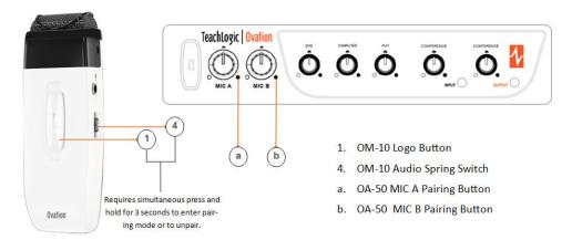
• If using two OM-10 microphones in the same room, one must be paired to the MIC B channel to avoid interference. Watch the how-to video on <u>teachlogic.com/resources</u>.
