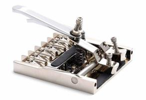
The **Duesenberg Multibender** enables you to play authentic sounding pedalsteel licks on nearly every normal electric guitar or lapsteel with a flat top. You can raise or lower Individual strings from 1 to 3 half tones (depending on the string gauge used) by pressing with the palm of the right hand on one or more of the multibender's levers, which is normally done with a foot pedal or knee lever on a pedalsteel guitar.
