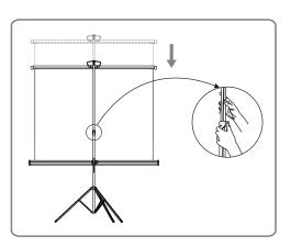
Adjust the height of the bottom casing using the locking handle.
